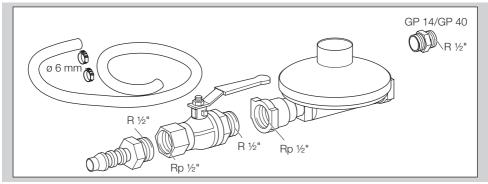
Pressure reducer, manual valve, hose (length = 2 m), 2 hose clamps, R 1/2" double nipple for GP 14/GP 40, to connect the gas combination control CG to the gas supply, Order No.: N52600025
