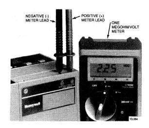
Move the flame detector and sight pipe (if not permanently attached to the burner/boiler) to view the flame from various positions. Allow a few seconds for the meter reading to stabilize. A maximum steady microamp or voltage reading is desirable. The flame signal must be above the minimum acceptable level for the flame safeguard control and associated amplifier as indicated in Table 1.
