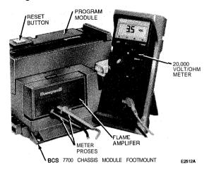
Fig. 9c—Measuring flame signal voltage of 7900 SERIES controls.
