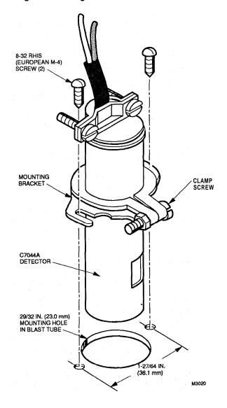
The C7044 is mounted in a 29/32 in. [23.0 mm] holeinthe blast tube. The mounting bracket is fastened to the blast tube with 2 screws on 1-27/64 in. [36.1 mm] centers.
