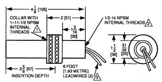
DIN APPROVED C7035A1064 HAS I-11 BSP,P1 INTERNAL THREADS.
