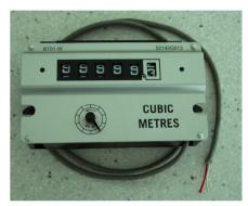
The pulse output provides a pulse every 1 cubic metre (m³) registered by the meter. For lesser values an optical sensor can be used to detect the rotation of the direct drive pointer every 0.05 cubic metres (m³) registered by the meter.
