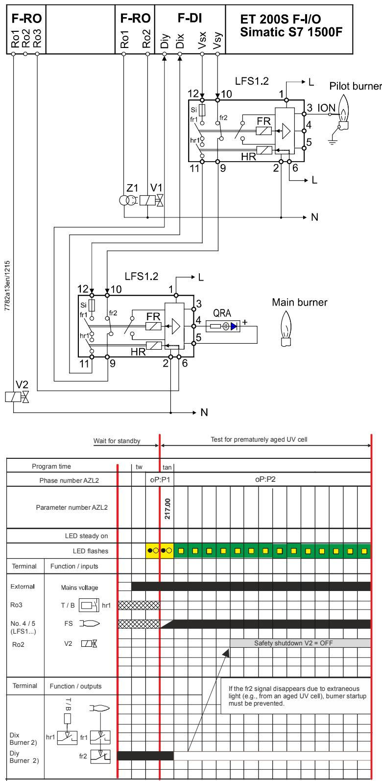
In the case multiflame supervision with a pilot burner, a fail-safe PLC performs the central control function (the example shown uses a Simatic S7 1500F and input / output modules ET 200S F-I/O).
