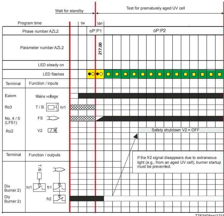
The test mode switchover for the burner 1 flame safeguard is inactive (terminal 6 is permanently connected to phase conductor L).
