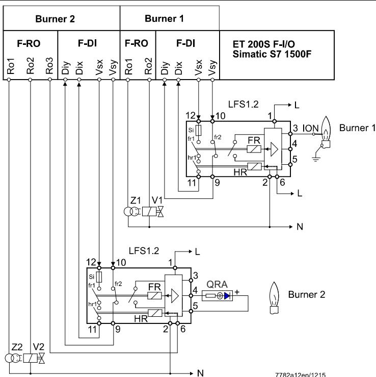
In the case of multiflame supervision, a fail-safe PLC performs the central control function (the example shown uses a Simatic S7 1500F and input / output modules ET 200S F-I/O).
