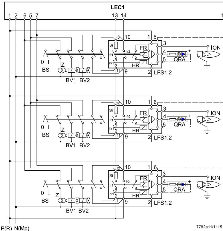
As with dual supervision, the control contacts of the flame relays of all flame safeguards must be connected in series in the case of multiflame supervision.
