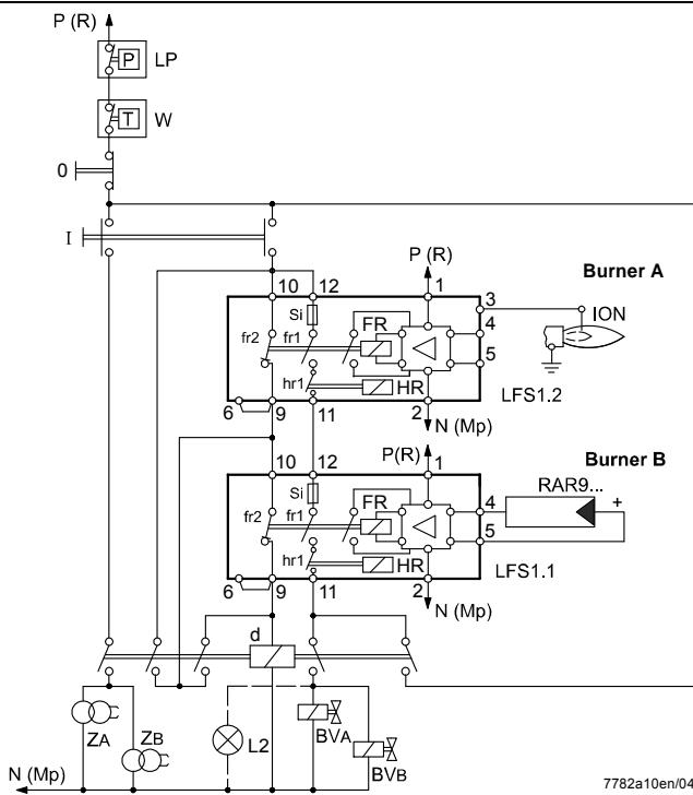
With this type of supervision, too, the burner can be started only if the flame detector test or flame simulation test has been successful. This means that **neither** of the 2 flame safeguards may detect a flame signal during burner off times. When the burner is started up, the detector test will automatically be interrupted. When button (I) is pressed, relay (d) is energized via circuit path 9...10 of the flame relays, which is still closed, thus switching on the ignition of both burners.
