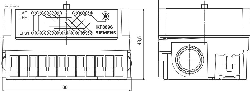
When replacing LAE10 and LFE10 with LFS1, adapter KF8896 ensures that the height can be adjusted mechanically and that the terminals are assigned correctly.
