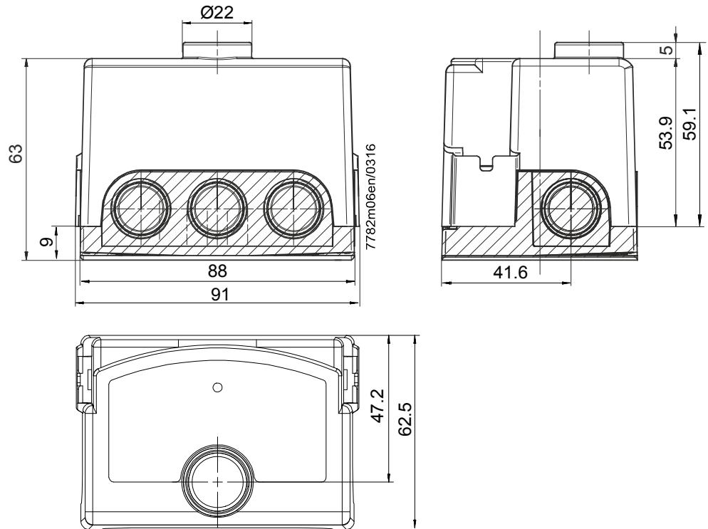
Plug-in base AGK11.7 with separating plate element (shown in green)
