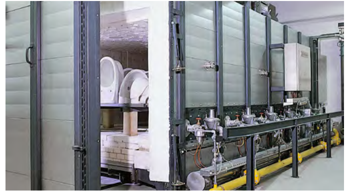
Ceramics industry: intermittent shuttle kiln
