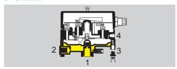
The pressure switch DG switches in the event of increasing or decreasing pressure. Once the set switching point is reached, a micro switch is activated in the DG which is designed as a change-over contact.
