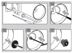
The spark electrode and flame rod can be removed without having to dismantle the burner chamber.
