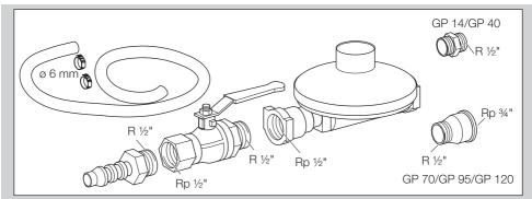
Pressure reducer, manual valve, hose (length = 2 m), 2 hose clamps, R 1/2" double nipple for GP 14/GP 40, R 1/2-Rp 1/2" reducing fitting for GP 70-GP 120, to connect the gas combination control CG to the gas supply, Order No.: N52600025
