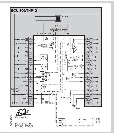
In order to ensure post-cooling, the heater constantly requires 230 V AC.
