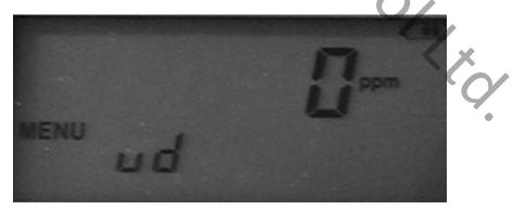
"Oppm ud (ud=under)" will display leaks in steps. The steps are Oppm, ud 500ppm, ud 1000ppm, ud 3000ppm, ud 5000ppm, ud 9999ppm
