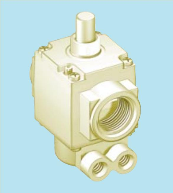
**Valve with thermoelectric safety device and pilot outlet with flow adjustment screw. Interruption of main gas flow while pilot is established.**
